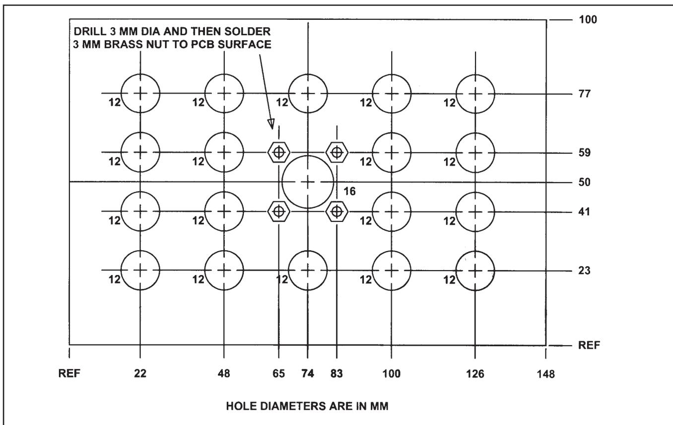
Figure 4. Lower PCB drilling details
