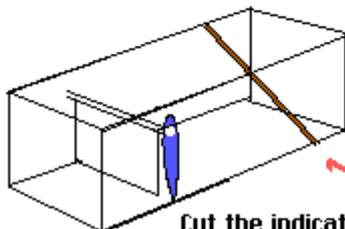
1" from the end of the tube box thread a wooden skewer through each corner as shown and glue in place to prevent the box collapsing.
