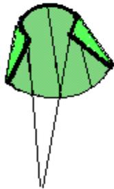
Due to the round shape, the bridle pulls the top of the circle in and the lower flares out making the kite stable.
