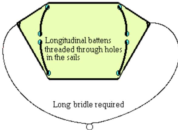
Spring-like battens prevent the leading edge of the canopy from collapse.
