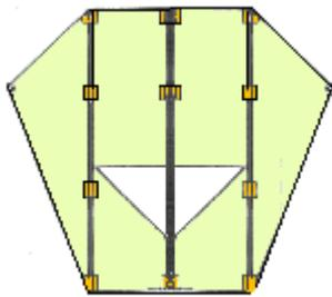
Frank Scott designed a flexible kite for Ray Holland to manufacture in 1967. The name Scott Sled is the title for the kite, registered to the company. The original size 40 inches by 35 1/2 inches. Three spars and a triangular vent are used. Colour of Polyethylene sail is yellow.
