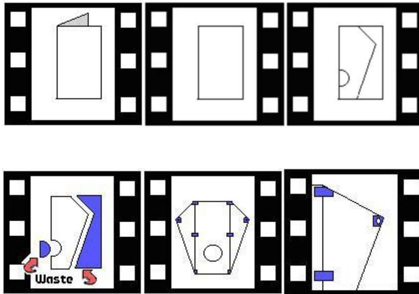
Remove the waste and unfold the kite pattern. Lay the kite on a flat surface. Place the two spars on the pattern as shown and stick down with adhesive tape at three points. Top, centre and trailing edge. Reinforce the two keel tips for the bridle line with a Band-Aid, folded so the adhesive is on both sides of the keel tip.
