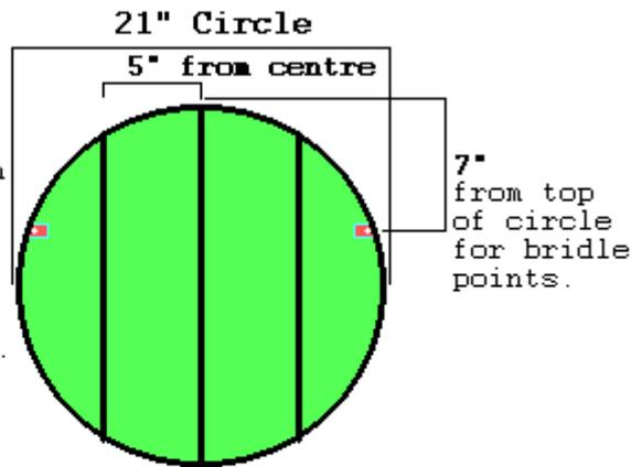
Three longerons are used 21" long and trimmed to fit the circle. Each longeron is held in place with adhesive tape in three places, top, centre and bottom of circle.
