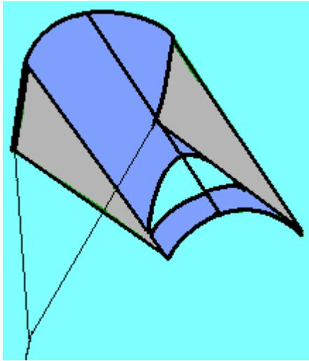
Scott retained the three spar (spine) of the original design. The centre spar was used to stiffen the flexible canopy to prevent the the leading edge of the canopy from folding and causing the kite to collapse. The sides were made parallel instead of the windsox taper that Allison incorporated in his design. A triangular vent was added, this force high-pressure air from below the sail into the turbulent airstream above the sail, serving to stabilise the Sled's flight.
