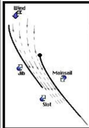
This is similar to the slot effect of the jib on a sailing boat that concentrates the airflow over the leeward side of the mainsail and causes it to accelerate.
