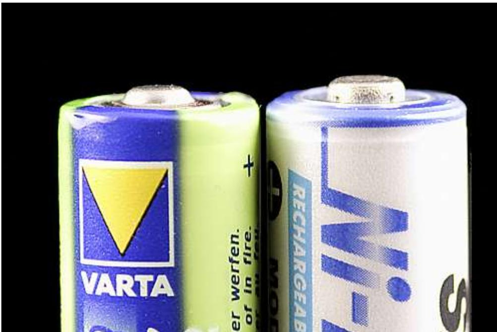
The second photograph shows how the Varta battery body is 1mm shorter than normal. If you look carefully you will see the Sanyo body is just a little longer than the Varta. Overall the Varta battery is the same size (shorter body, but longer charging nipple) so it can fit into devices that use AA batteries.
